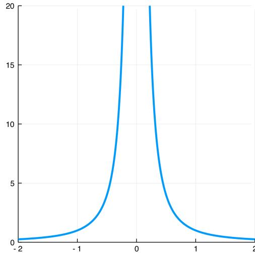
This is an example of a function *diverging to infinity*: we say  $f$  diverges to infinity at  $c$  if we can make  $f(x)$  as large as we like by taking  $x$  sufficiently close to  $c$
