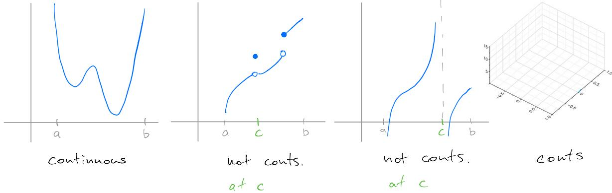
the points of discontinuity are points  $c$  where  $\lim_{x \rightarrow c} f(x)$  doesn't exist or where  $\lim_{x \rightarrow c} f(x) \neq f(c)$
