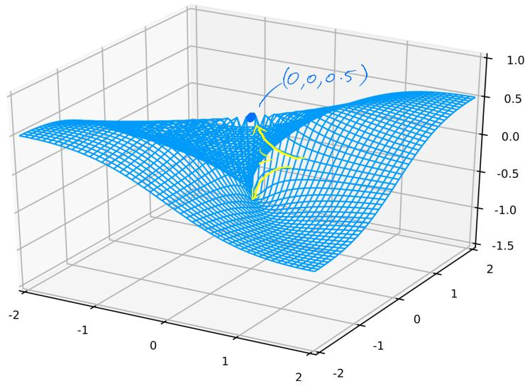
intuitively: not continuous at  $\underline{0}$  - there is tearing
